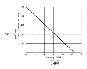
The curve above shows that with a 100 foot change in head, the capacity varies only 2 gallons per minute. You get a virtually constant flow over wide pressure variations to ensure reliable system operation.
